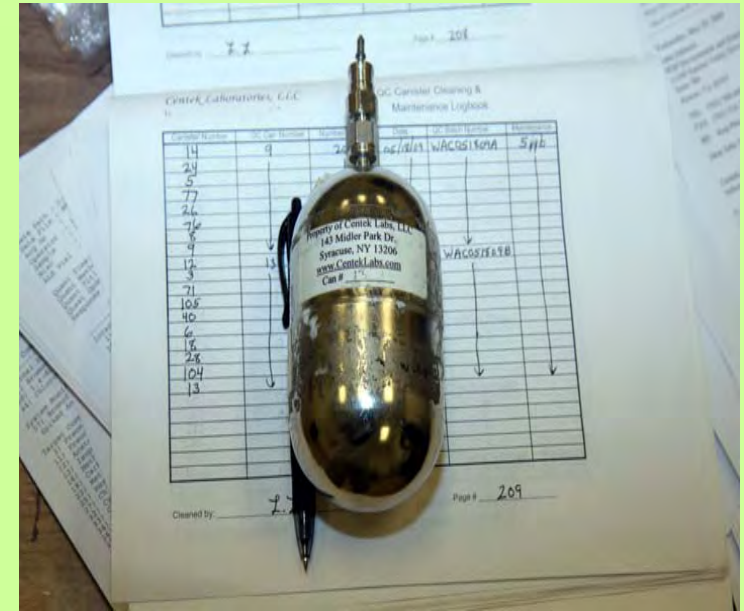
Example of stainless steel container used for air sampling..
