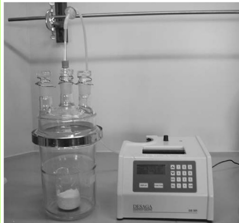
Figure 1. Sampling of headspace above GyP on a TENAX-TA® tube.
